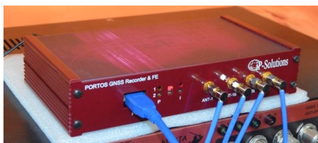
Ninja A8-R6-Q14-U3 CRPA simulator And PORTOS A4-LS-R4-U3 front end
