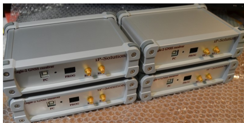
Eagle-2 A2-L1-R2-U2 with two synchronized RF channels.
